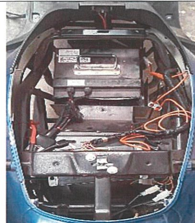
5. DO DRIVE Battery Location
